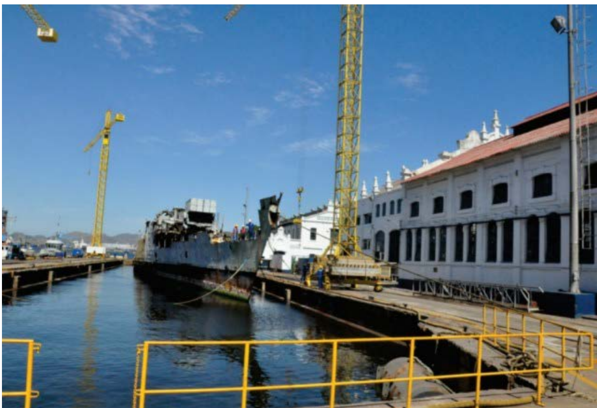
Photo 4 - Diagonal displacement along the dyke, with the protruding bow to the chassis of the crane
