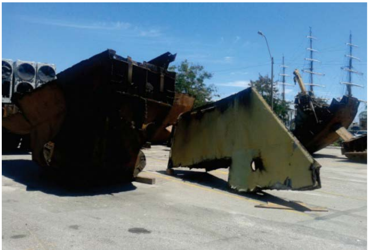
Photo 9 - Large blocks and equipment removed from the ex-D30 and displaced by CFM's CavMec, so that they could later be dismantled outside the dike
