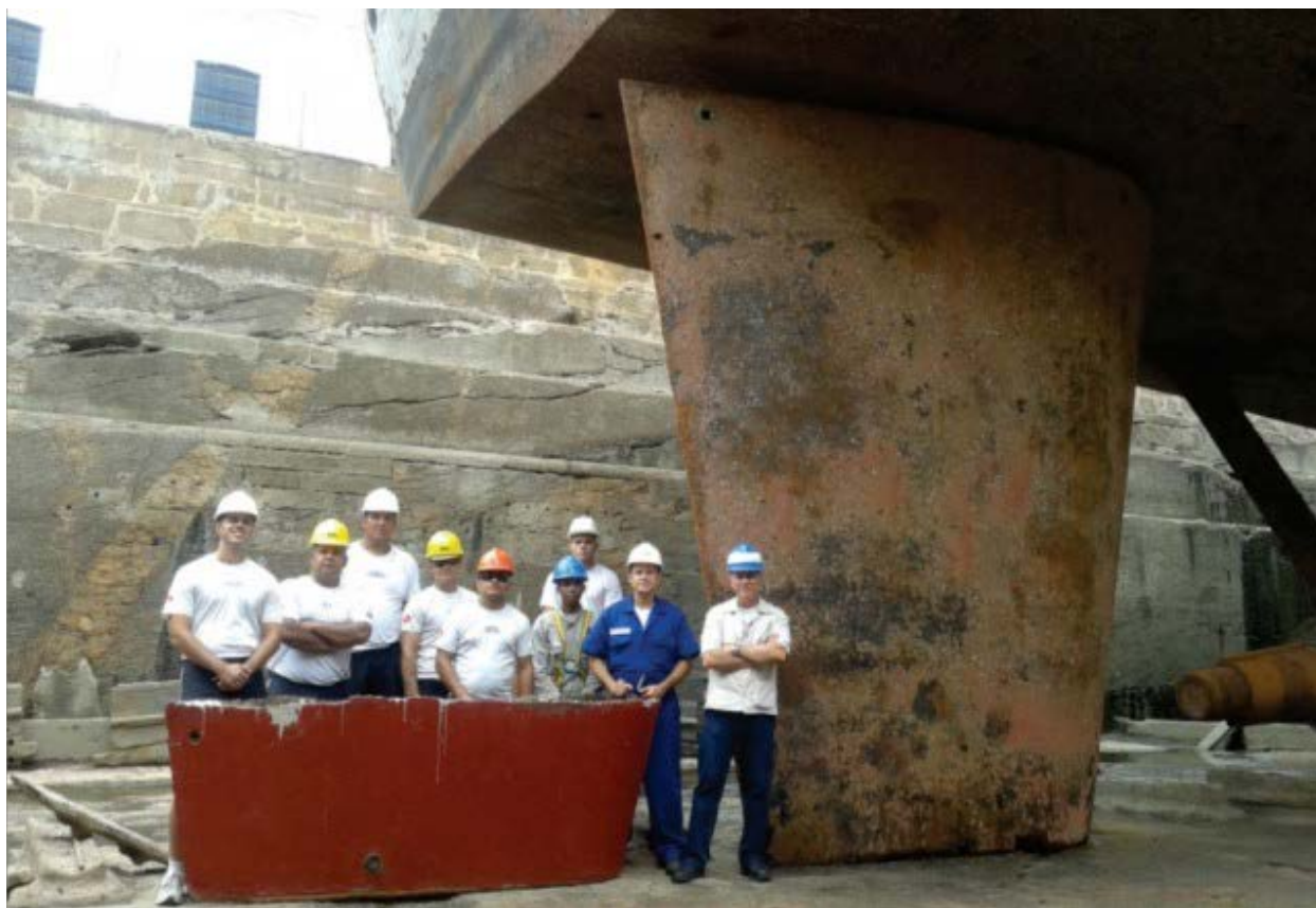
Photo 6 - Detail of the part of the rudder that was sectioned while the hull was still floating and also of the performance of the rudder as a "fortune column" supporting the stern
